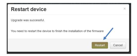
9. The upgrade is now complete. Once the device has finished rebooting, check that the version has been installed on the Home page of the Cloudgate under System Information.
