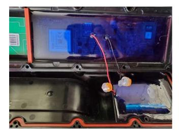
• Using wire snippers, cut both the red and black wires from the Scotchlok connectors. To ensure there will be plenty of wire for connecting the new battery, snip the wire as close to the Scotchlok connector as possible.
